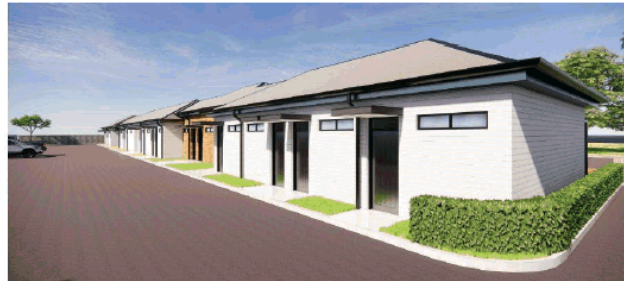
The detail of the rear to the vehicle area where design development is expected to reduce the dominant road surface and provide for personal safety. The Weathertex classic 200mm boards are acceptable while the White clour needs to be reconsidered as a Warm White and the gutter colour reconsidered as Monument is not acceptable in the HCA.
